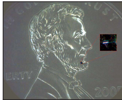
Dartmouth's microbot is untethered and controllable, yet 200 of them could fit in line across the top of an M&M. Photo courtesy of the Donald Laboratory.
